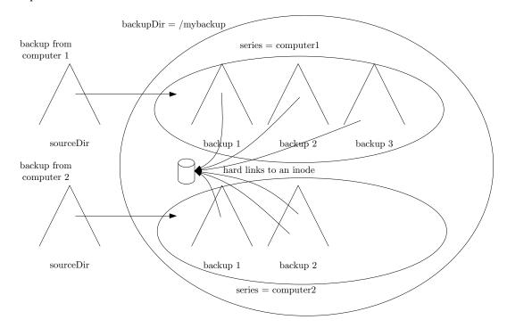
Imagine you have two computers you want to backup on one file server via NFS. If you only want to backup on an external disk (eg. usb or esata), you should also read the following to understand the basic parameters. See section 4.14.6 how to configure NFS properly — you must have write access to the directory where you want to save your backup. If you are root, you should have root permissions on this mounted directory.
